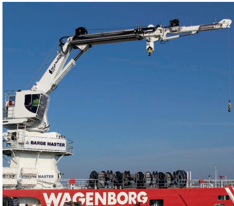
CUSTOM CRANE: The motion compensating BM-T40 crane went from the drawing board to ship's deck in just 18 months.
