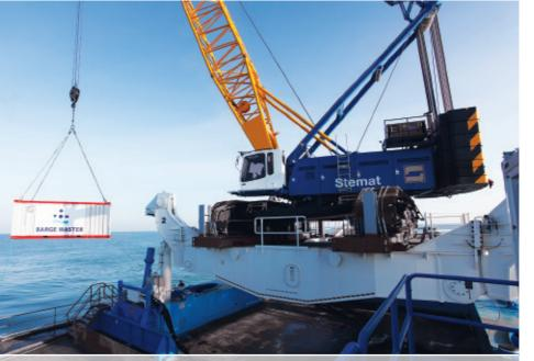
BM-T700 motion compensating platform in use as a crane platform
