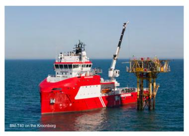
The BM-T40 is working for Shell/NAM since 2015 on the W2W vessel Kroonborg. By using a dedicated vessel Shell/NAM where able to decommission all there platform cranes. The BM-T40 outperformed the initial expectations, making it possible to work 330 days a year. This resulted in a second W2W vessel, the Kasteelborg.
