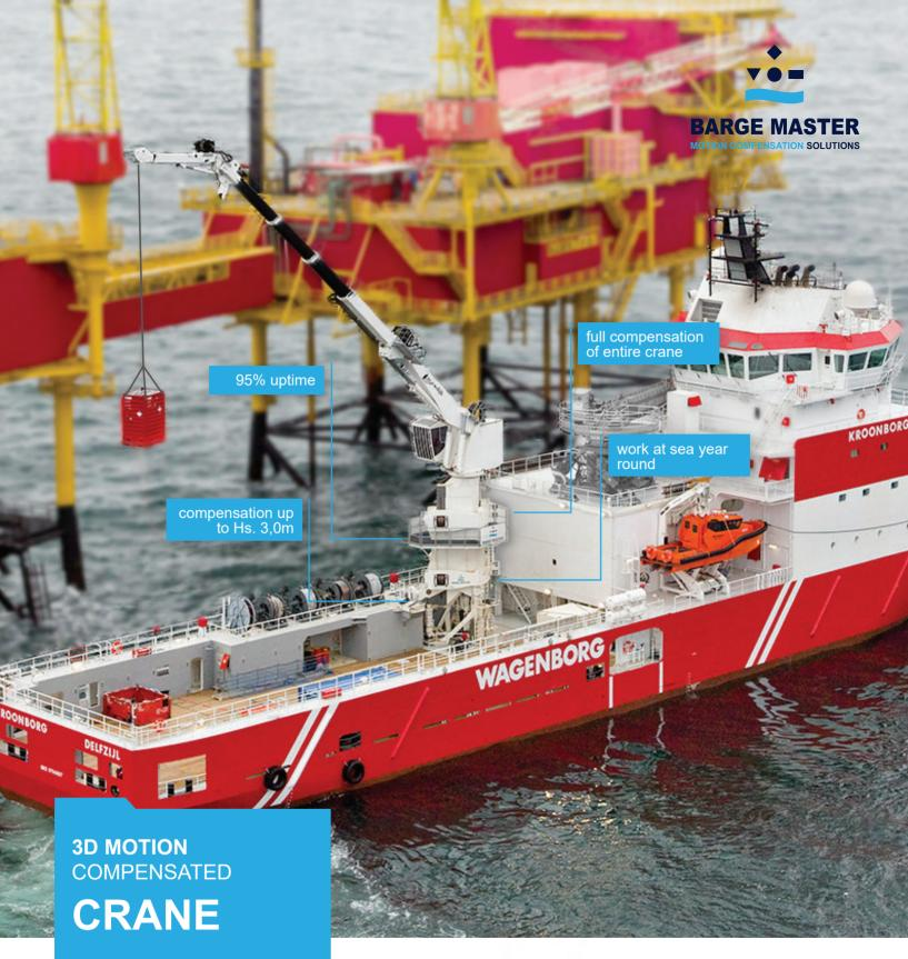
The Barge Master Motion Compensated Crane enables controlled lifting operations with a high crane capacity, making it possible to work at sea almost year-round. It has proven to increase workability in the North Sea from 180 to 330 days.
